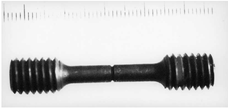
Fig. 1. Standard tensile V-notch sample.
